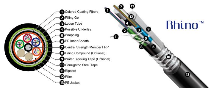
LP-OC04XX Fiber Optical Cable with Loose Tubes, Double PE Jacket, Central Strength member FRP, Glass yarns, Dry Water Block Cable Core and Ripcord.
