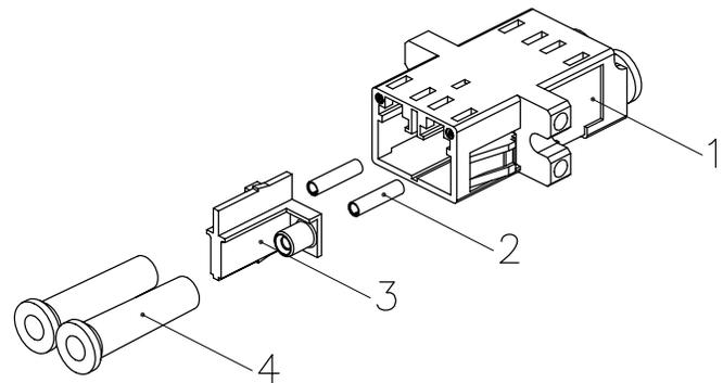
1. Housing : Polycarbonate, UL94V-0
