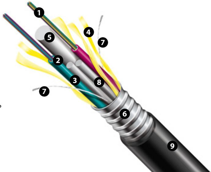
**LP-OC20XX** Fiber Optical Cable with Loose tube, Single PE Jacket, armored with two steel wires strength members, laminated steel tape, Dry Water Blocking tape and Ripcord.
