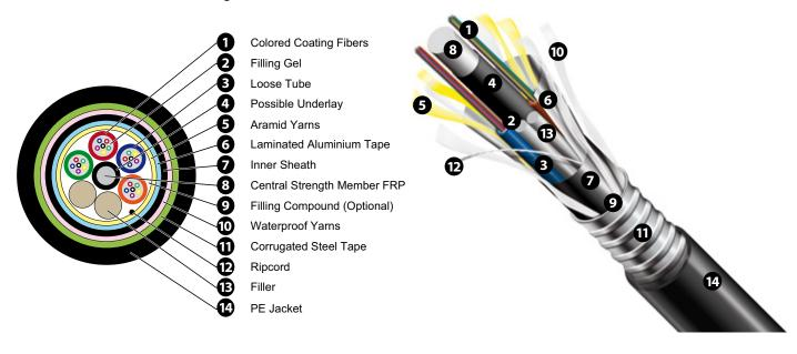
LP-OC07XX Fiber Optical Cable with Loose Tubes, Double PE Jacket, self supporting, Figure 8, central steel wire, messenger wire, laminated aluminum tape for strength, Dry Water Block Cable Core and Ripcord.
