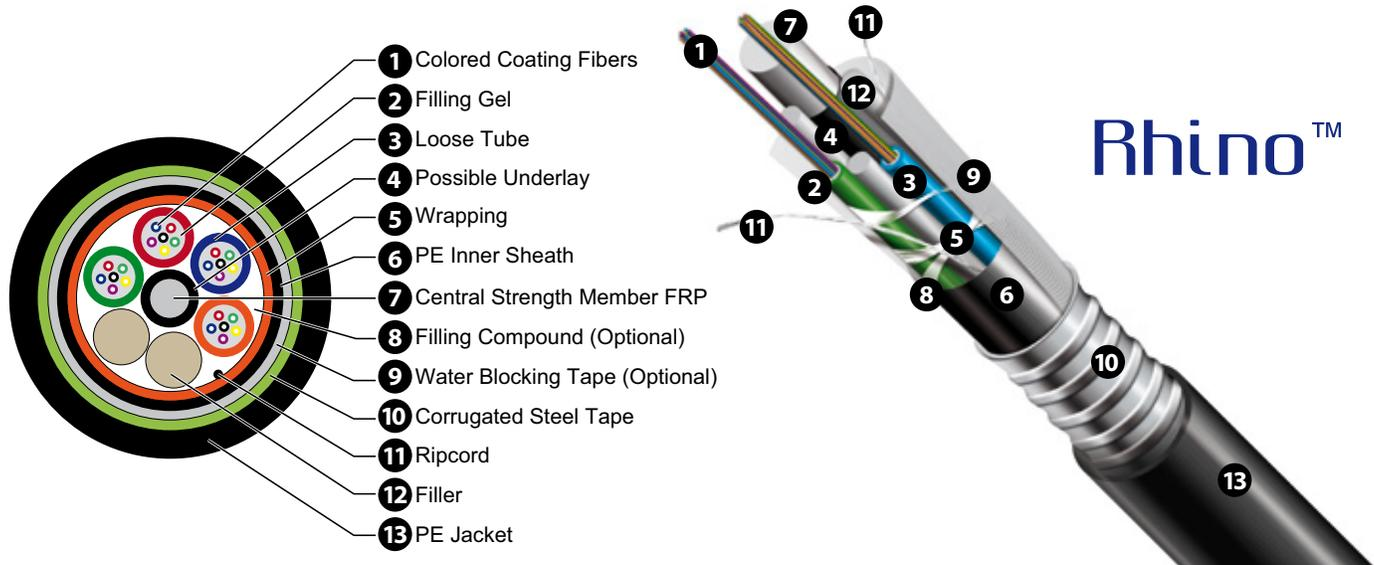
**LP-OC04XX** Fiber Optical Cable with Loose Tubes, Double PE Jacket, Central Strength member FRP, Glass yarns, Dry Water Block Cable Core and Ripcord.
