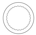
Inner wall with longitudinal ribs to guide the airflow
