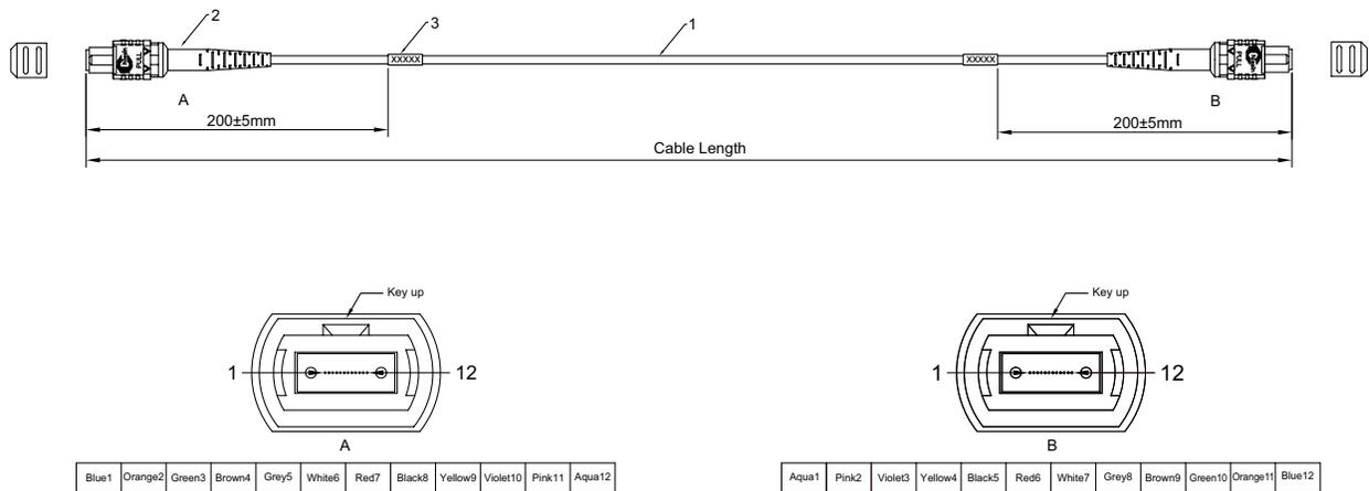
Fiber Optic patch Cord MPO/PC-MPO/PC 12 Fibers Multimode
