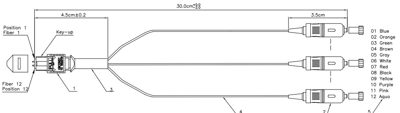
1. Connector type: Guide pin MTP® multimode, male connector, low loss
