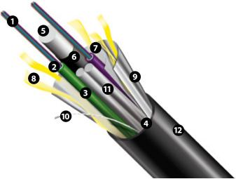
**LP-OCO8XX** Fiber Optical Cable with Loose Tubes, Single PE Jacket, self supporting, Figure 8, Central steel wire, messenger wire, Laminated Aluminum tape and Ripcord.
