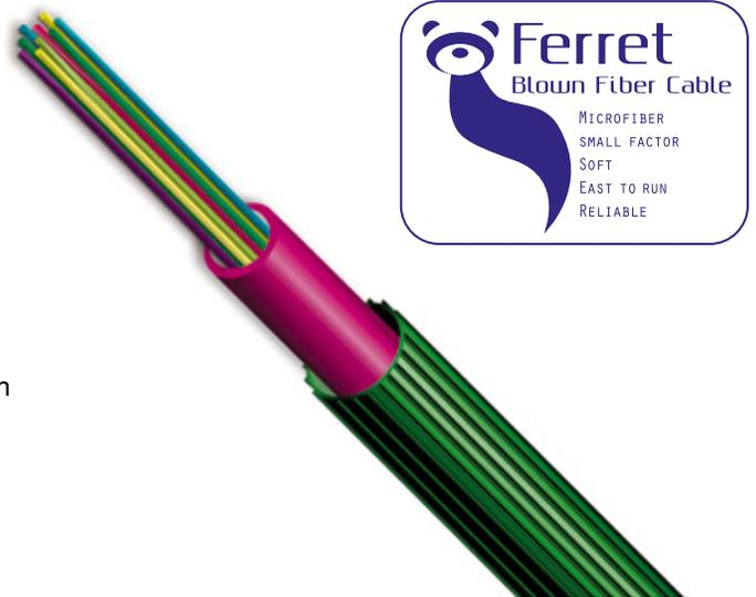
**LP-OC81XX** Ferret™ Series, Blown Fiber Optical Micro Cables with Loose Tubes Single PE Jacket, central strength member of FRP, Peripheral water blocking yarns, Dry water block cable core (12-288 cores).
