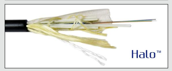
Loose tube cables are the most widely used cables for outside plant trunks because it offers the best protection for the fibers under high pulling tensions and can be easily protected from moisture with water-blocking gel or tapes.
