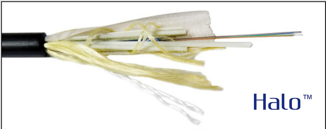
Loose tube cables are the most widely used cables for outside plant trunks because it offers the best protection for the fibers under high pulling tensions and can be easily protected from moisture with water-blocking gel or tapes.
