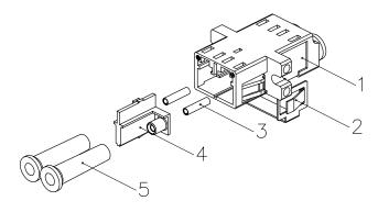
1. Housing: Polycarbonate, UL94V-0
