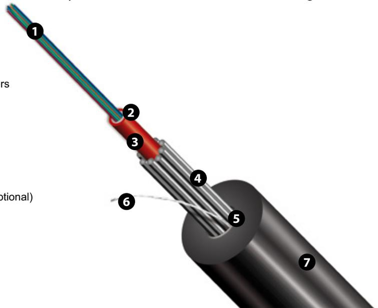
**LP-OC22XX** Fiber Optical Cable with central Loose Tube, Single PE Jacket, layer of galvanized steel wires strength member, bonded steel tape, water blocking tape and Ripcord.
