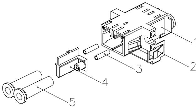
1. Housing : Polycarbonate, UL94V-0
