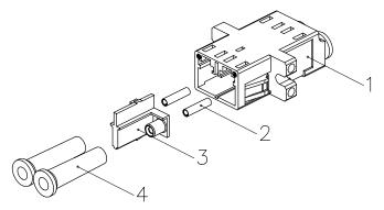
1. Housing: Polycarbonate, UL94V-0
