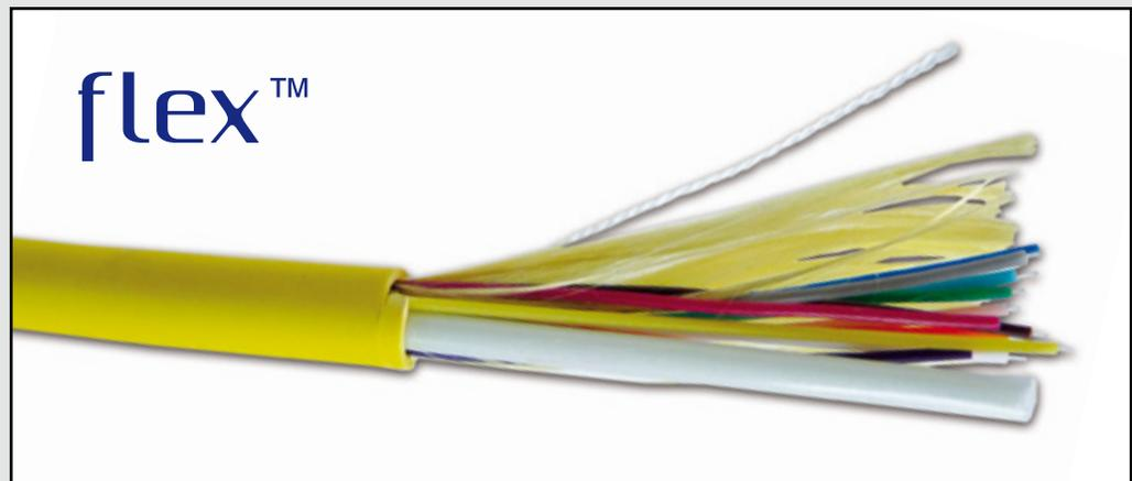
Distribution cable is the most popular indoor cable, as it is small in size and light in weight. They contain several tight-buffered fibers bundled under the same jacket with Kevlar strength members and sometimes fiberglass rod reinforcement to stiffen the cable and prevent kinking. These cables are small in size, and used for short, dry conduit runs, riser and plenum applications.
