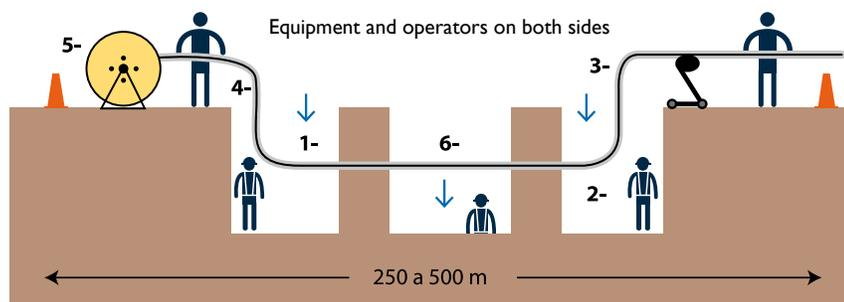
The inner diameter of the duct should be much larger than the diameter of the cable to reduce friction and lower the installation tension force.
