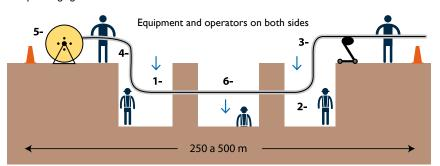
The inner diameter of the duct should be much larger than the diameter of the cable to reduce friction and lower the installation tension force.
