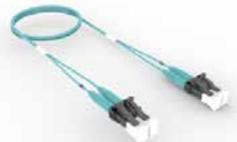
PATCH CORD OM4 LAZRSPEED 550 LC TO LC FIBER PATCH CORD, 1.6 MM DUPLEX, RISER, 60 FT
