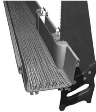
Fixture protects cables during cutting of sidewall
