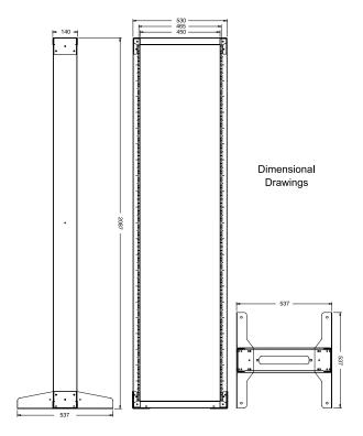
Our multi use two post rack is a cost and space effective way to install a variety of 19" equipment. Intended primarily for patch panels or network switching equipment, the two post rack can also be fitted with shelves to support equipment.
