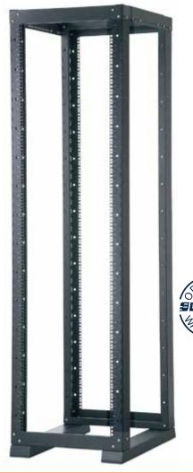
The LP-R712XXXXX 7000 Series of 4-Post Open Frame Racks constitute a very economic solution for server, network, audio and telecommunication equipment rack mounting. The Frames come in four (4) Sizes: 27U, 37U and 42U, and in three (3) depths: 600mm, 800mm and 1000mm. Width is 600mm to allocate the 19" EIA standard size width of rack mounted equipment.
